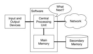
Figure 1.3: Hardware Architecture
